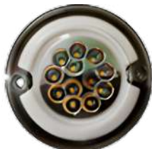
REAR COMBINATION LAMP ASSY DRL ROUND TYPE (INDICATOR / REVERSE FUNCTION) REFLECTOR BASED
